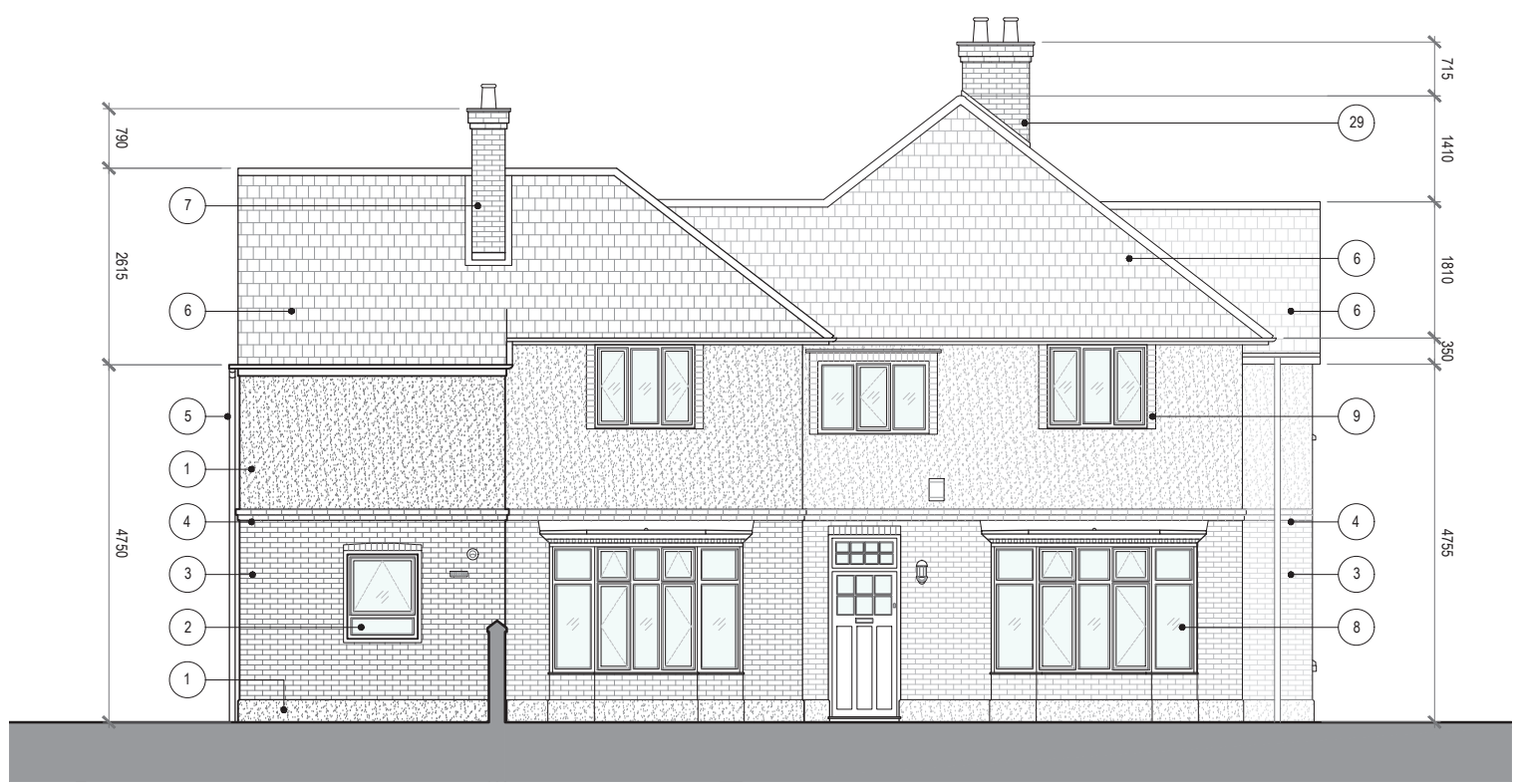
existing south elevation
